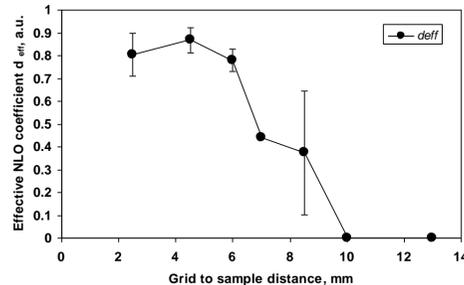
Figure 2 Effective NLO coefficient as a function of grid to sample distance
