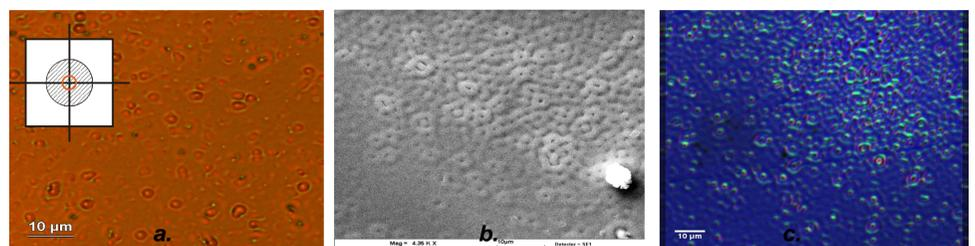
Figure 8 Images made using (a) optical microscope, (b) SEM and (c) second harmonic microscope
