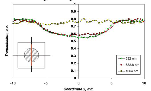
Figure 7 Transmission at 532, 632.8 and 1064 nm of sample poled at grid voltage 1.5 kV
