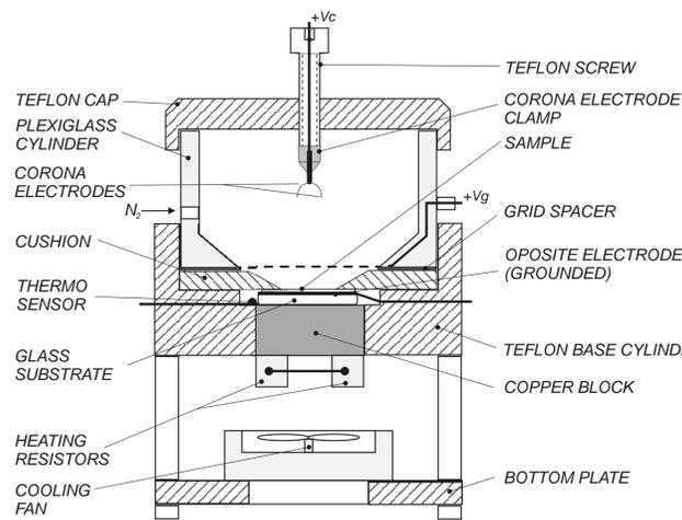
Figure 1 The principal scheme of corona discharge device
