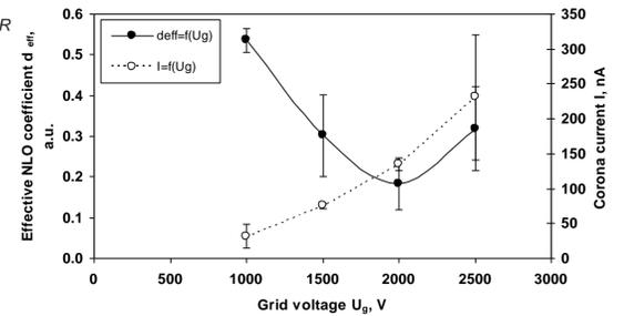
Figure 5 Effective NLO coefficient and corona current as a function of grid voltage
