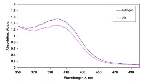
Figure 4 Absorption spectra for samples poled in air and nitrogen atmosphere
